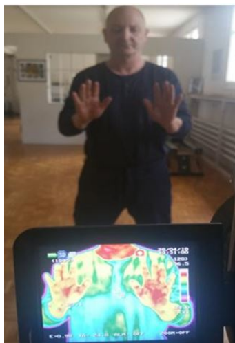
Figure 1: Measuring principle applying an infrared camera to monitor probands temperature distribution of the body part under test, in this case the hands of the seiki therapist Mr. Damljanovic.
